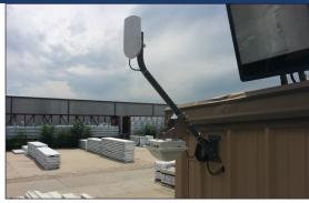
ePMP module and WLAN Access Point
